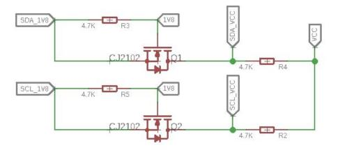
This is a typical Bi-directional level shifter circuit to connect two different voltage section of an I<sup>2</sup>C bus. The I<sup>2</sup>C bus of this sensor use 1.8V, if the I<sup>2</sup>C bus of the Arduino use 5V or 3.3v, this circuit will be needed. In the schematic above, **Q1** and **Q2** are N-Channel MOSFET <u>CJ2102</u>, which act as a bidirectional switch. In order to better understand this part, you can refer to the <u>AN10441</u>
