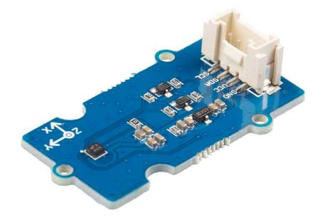
The Grove - 3-Axis Digital Accelerometer ±16g Ultra-low Power (BMA400) sensor is a 12 bit, digital, triaxial acceleration sensor with smart on-chip motion and position-triggered interrupt features. It can detect your movement posture, such as Walking, Running, Standing still.
