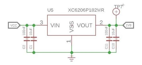
The typical voltage of BMA400 is 1.8V, so we use the  $\underline{XC6206P182MR}$  chip to provide a stable 1.8V. The input of XC6206P33 ranges from 1.8V to 6.0V, so you can use this module with your Arduino both in 3.3V and 5V.
