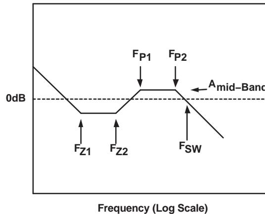
**Figure 25. Error Amplifier Frequency Response Straight Line Approximation**
