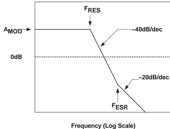
Figure 24. Power Stage Frequency Response Straight Line Approximation
