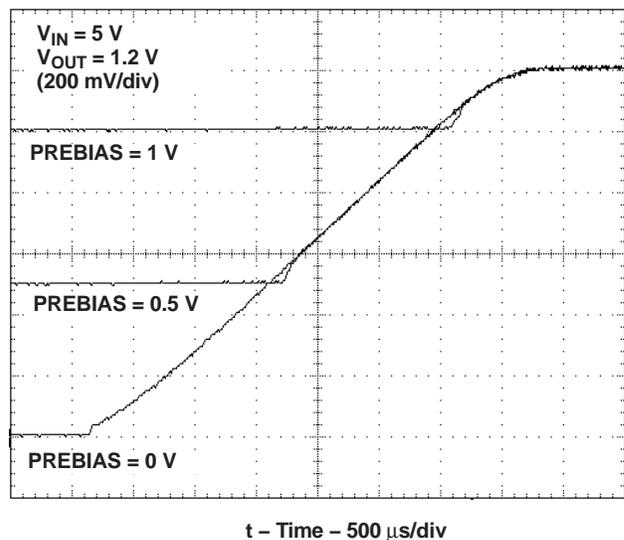
Figure 21. Startup Waveforms
