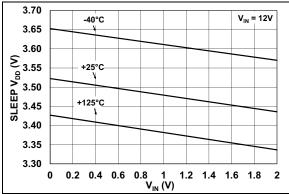
**FIGURE 7-17:** Average SLEEP  $V_{DD}$  Output Voltage vs. Current.
