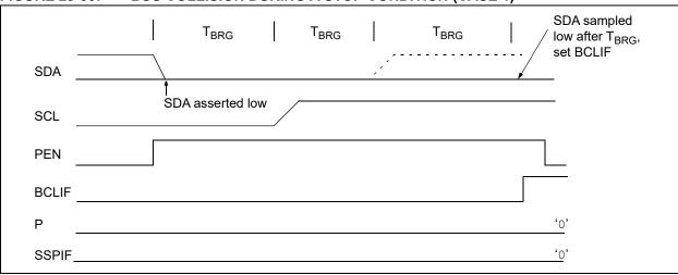
FIGURE 29-31: BUS COLLISION DURING A STOP CONDITION (CASE 2)
