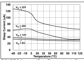
FIGURE 7-2: IQ vs. Temperature in Sleep Mode.
