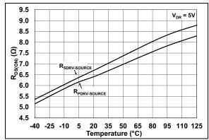
**FIGURE 7-10:** Sourcing Output Driver  $R_{DS(ON)}$  vs. Temperature.
