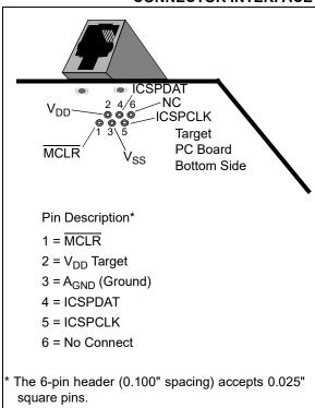
Another connector often found in use with the PICkit™ programmers is a standard 6-pin header with 0.1 inch spacing. Refer to Figure 31-2.
