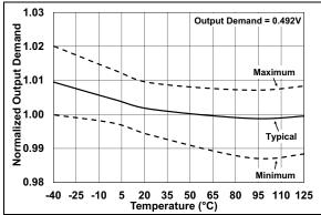
FIGURE 7-14: Normalized Output Demand vs. Temperature.
