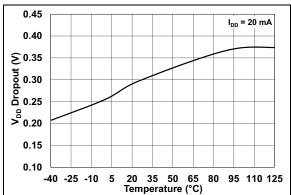
**FIGURE 7-6:** V<sub>DD</sub> Dropout Voltage vs. Temperature.
