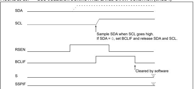
FIGURE 29-29: BUS COLLISION DURING A REPEATED START CONDITION (CASE 2)
