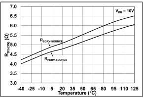
**FIGURE 7-8:** Sourcing Output Driver  $R_{DS(ON)}$  vs. Temperature.
