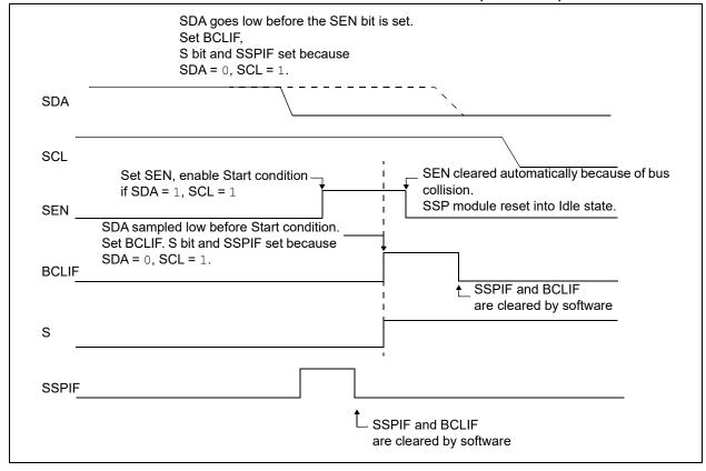
FIGURE 29-26: BUS COLLISION DURING A START CONDITION (SCL = 0)
