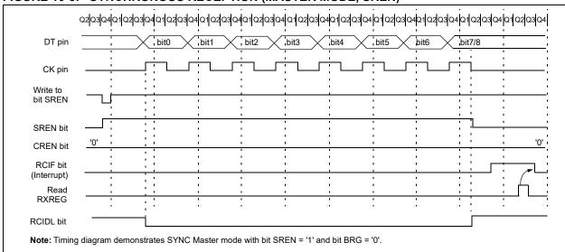
FIGURE 10-3: SYNCHRONOUS RECEPTION (MASTER MODE, SREN)
