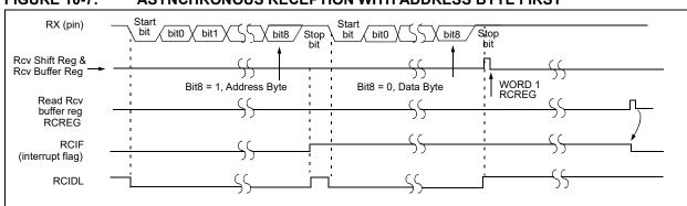
Note: This timing diagram shows an address byte followed by an data byte. The data byte is not read into the RCREG (receive buffer) because ADDEN was not updated and still = 0.
