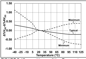
**FIGURE 7-15:**  $V_{DD}$  vs.  $AV_{DD}$  Temperature Drift Tracking.
