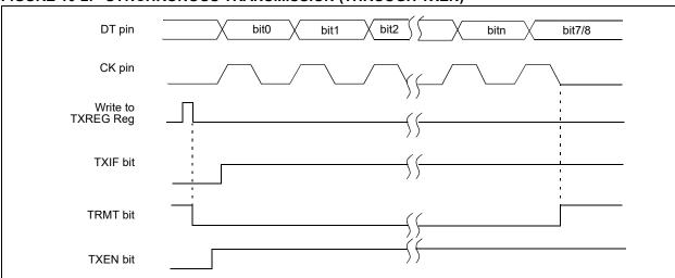
FIGURE 10-2: SYNCHRONOUS TRANSMISSION (THROUGH TXEN)
