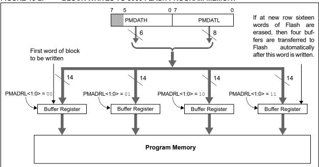
FIGURE 18-3: FLASH PROGRAM MEMORY LONG WRITE CYCLE EXECUTION
