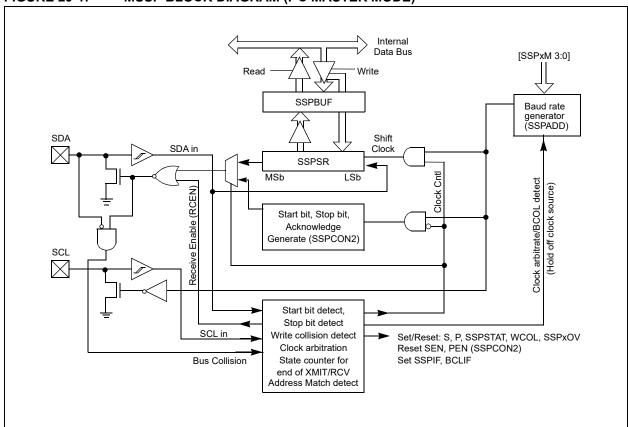
FIGURE 29-2: MSSP BLOCK DIAGRAM (I<sup>2</sup>C SLAVE MODE)
