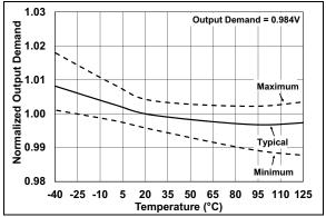
**FIGURE 7-13:** Normalized Output Demand vs. Temperature.
