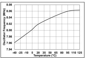
**FIGURE 7-12:** Oscillator Frequency vs. Temperature.
