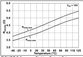
**FIGURE 7-9:** Sinking Output Driver  $R_{DS(ON)}$  vs. Temperature.
