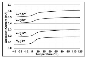
FIGURE 7-1: I<sub>O</sub> vs. Temperature.
